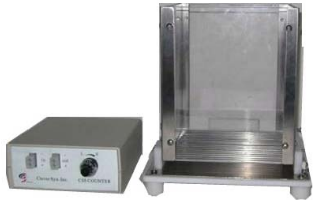
Parallel Rod Apparatus and Foot Slip Counter
